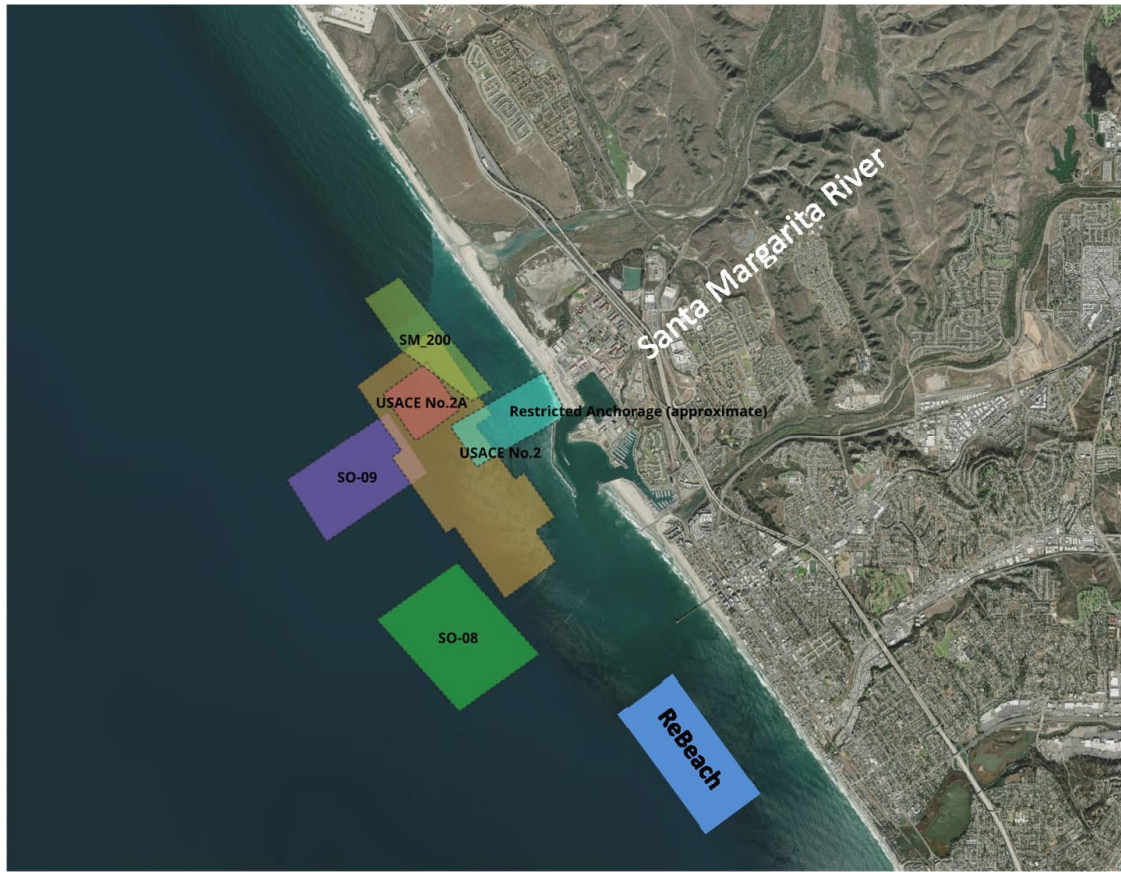
Figure 8 - Previous and Proposed Borrow Areas at Oceanside Harbor and the Santa Margarita River. Borrow area SM-1 (light green) was explored but not used for RBSP II. USACE Borrow 2A (orange) was dredged initially for San Clemente but discontinued due to gravel content. The proposed borrow footprint for the Oceanside Sand Nourishment and Retention Pilot Project (“ReBeach”) is shown in blue (GHD 2024).
