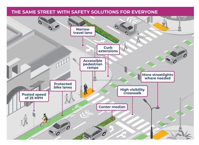
The data analysis performed for the Vision Zero Action Plan provides insights into the locations and nature of safety challenges across the region. The systemic implementation of proven road design features can target underlying crash causes, considering people driving, walking, biking, and rolling. For more information on safety solutions, see Appendix C.
