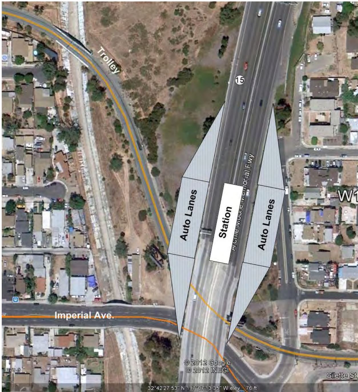
Figure 5 high resolution image showing the proposed moved auto – BRT lanes and station.
