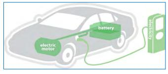
**Plug-in Hybrid Electric Vehicle (PHEV)** - Plugs into the grid and operates on electricity as well as an internal combustion engine.
