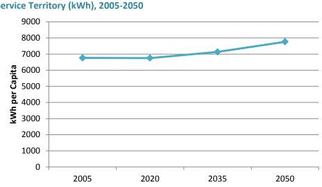
Figure 4-6: Existing and Projected Per Capita Electricity Consumption for SDG&E Service Territory (kWh), 2005-2050
