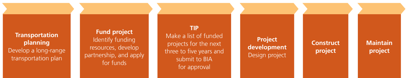
Figure 2.2 – Project development process
