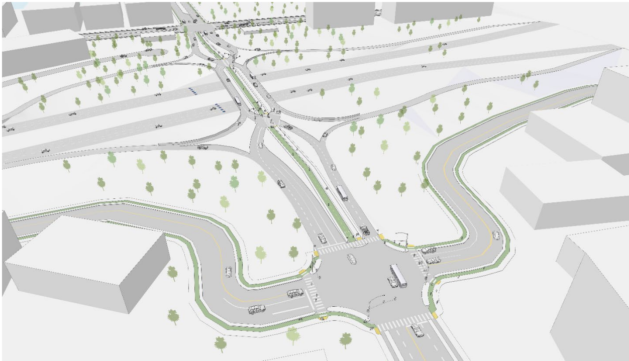
Conceptual rendering of the Diverging Diamond Interchange at Texas Street/Qualcomm Way and Interstate 8.
