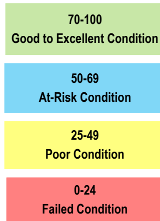
EXHIBIT 22. TYPICAL PAVEMENT CONDITION INDEX RANGES
